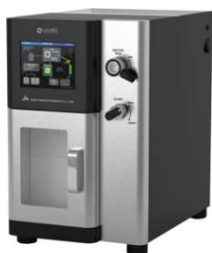
Recycling Preparative HPLC LaboACE LC-5060
