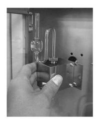
2) Slowly withdraw the siphon counter so as not to damage piping above the siphon box.
